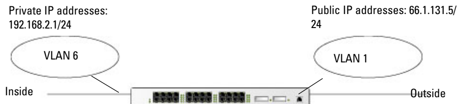
Figure 4 Example: Source NAT using Controller IP Address
